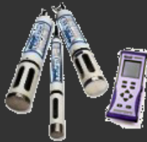
Multiparametric probes Water temperature, salinity, turbidity, pH, Chlorophylla, etc
